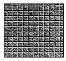
To calibrate instrument magnification use the following calculation where **A** represents the **distance in mm between limiting lines of the spaces measured** and **B** represents the **number of spaces measured**:
